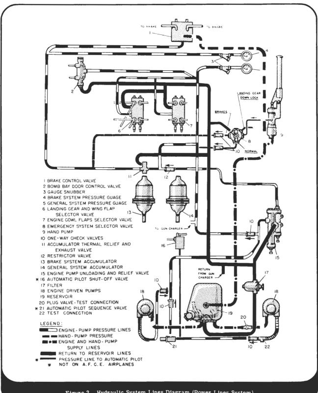
Figure 2 - Hydraulic System Lines Diagram (Power Lines System)
