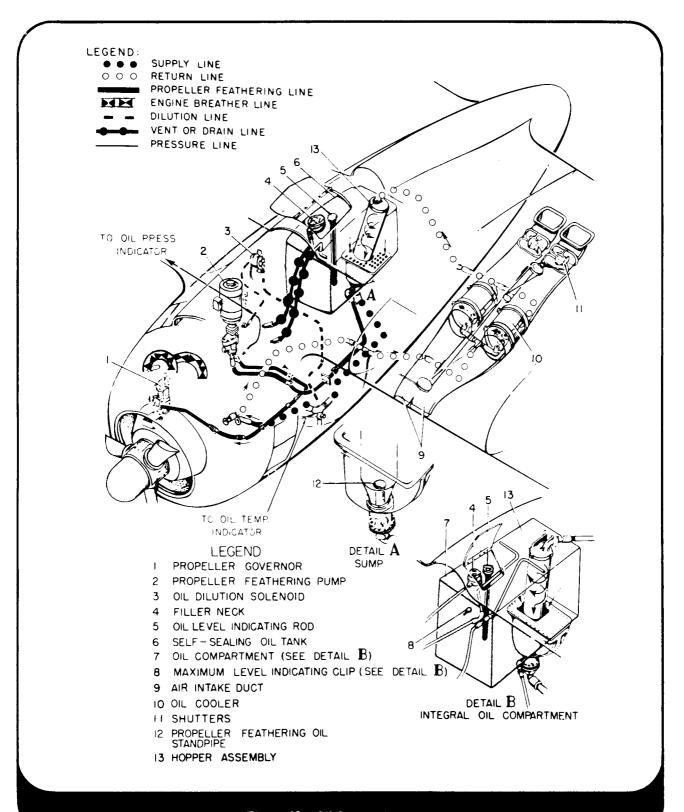
Figure 12 - Oil System Diagram
