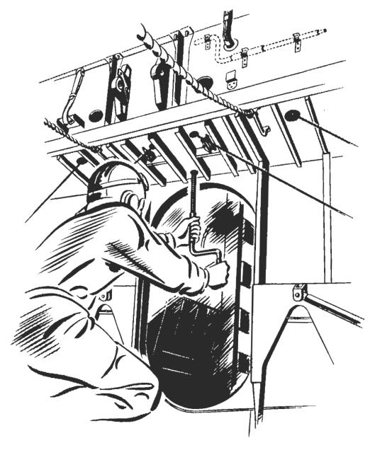
Figure 14 -- Wing Flaps Operation, Emergency
